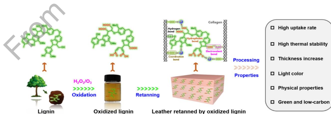
Figure 1. Proposed mechanism of lignin oxidation and its applications.
