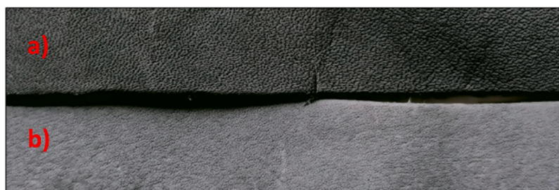
Fig. 6. Surface aspect of ED8-treated leather (a) compared to that of the not treated leather (b).
