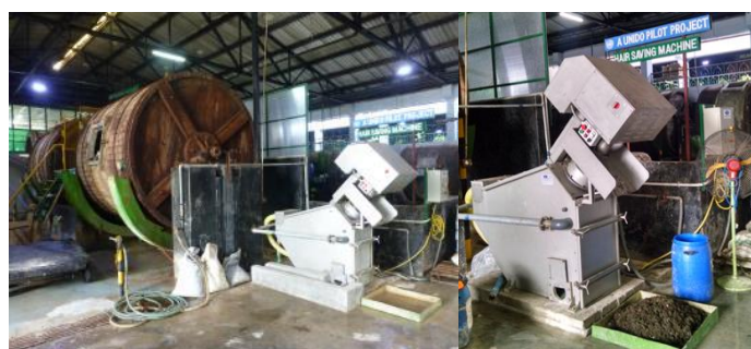
Figure 1 & 2: Hair saving screen installed within existing tannery
