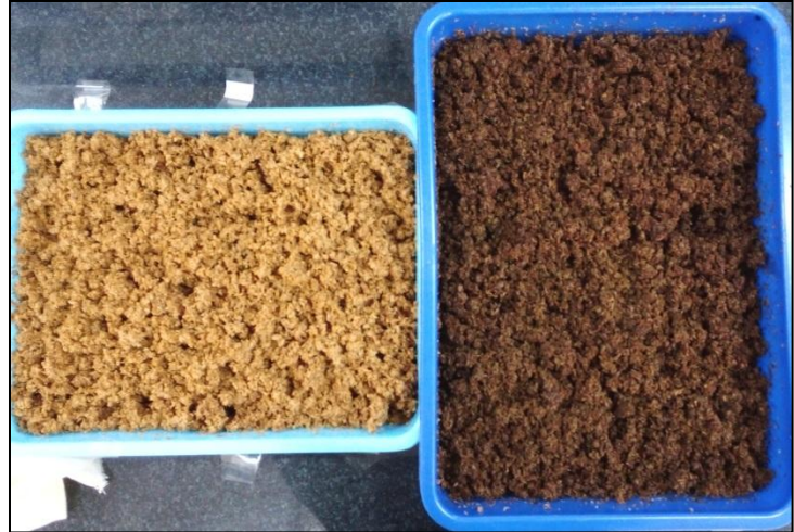
Fig. 1. SSF enzyme production on sterilised plastic trays; Image from left to right shows the changes in visual appearance of the wheat bran on first and last day of fermentation process
