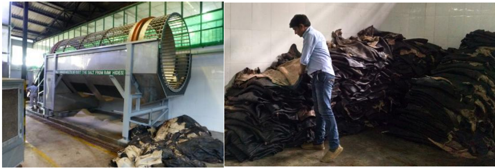
Figure 17: Desalting drum Figure 18: Raw hides after desalting
