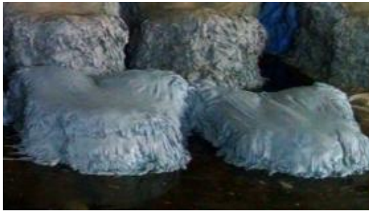
Fig16. Wetblue produced from chilled hide processing
