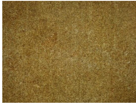
Figure 4: Fabricated composite from dechromed shavings
