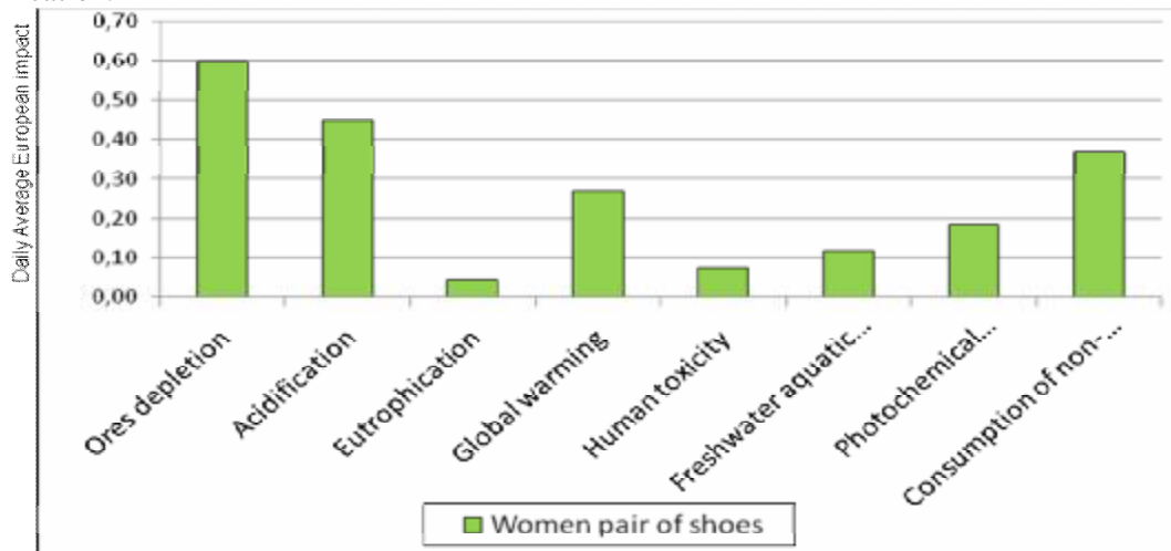
Fig. 1 Example of the impact of a pair of women's town pair of shoe (standardisation)
