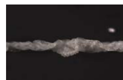
Fig. 5 Collagenic biopolymer extruded fibre, by optical microscopy (diameter 300µm)
