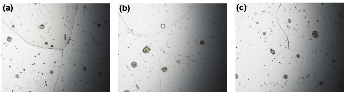
Fig. 8. Optical microscope images (at 100× magnification) of the produced iron metals using a) shavings char, b) buffing dust char and c) leather cuttings char.
