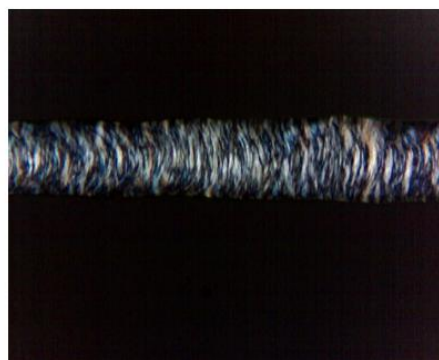
Figure 5. Polarizing optical microscopy image of a collagen fiber obtain from 20.8 wt% collagen.
