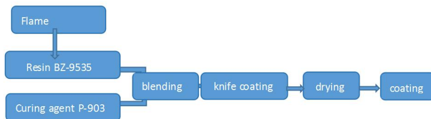
FIG. 1 flowchart of flame retardant PU coating preparation
