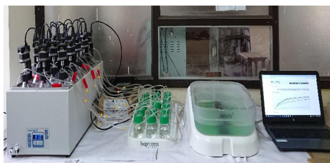
Figure.3 Automated methane potential test system II (AMPTS II) experimental set up
