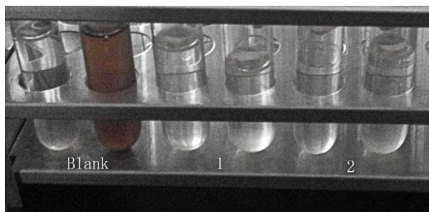
Fig.1 The S 2- elimination effect of enriched microorganisms (Blank is Na 2 S solution without the microorganisms; 1 and 2 are Na 2 S solution inoculated with the microorganisms. Test tube on the left side is Na 2 S solution without copper reagent and test tube on the right side is adding copper reagent)
