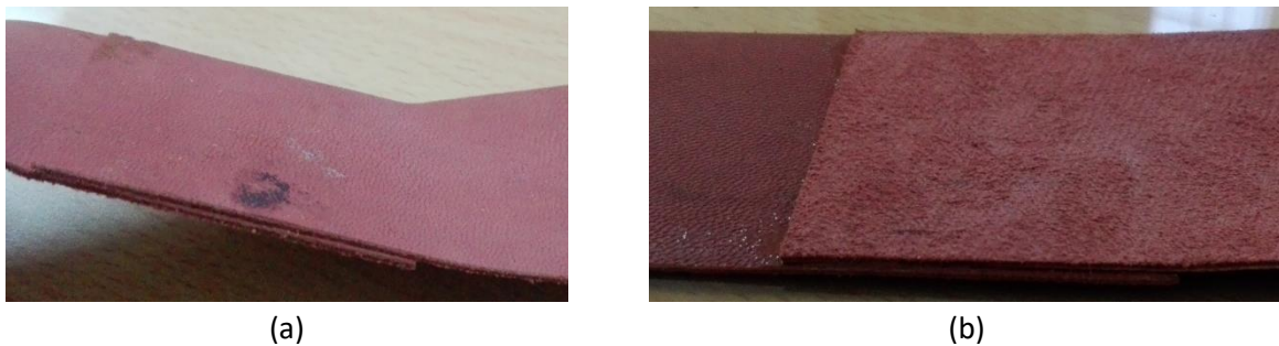
Figure 5: Bond formed by prepared adhesive (a) grain-to-flesh and (b) grain-to-grain
