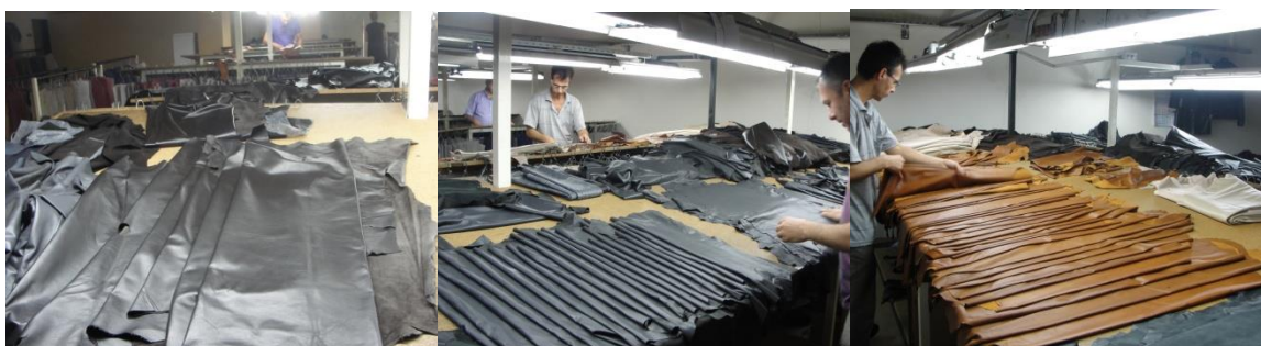
Fig.1. Assorting process in leather garment manufacture
