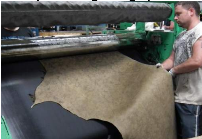
Grain patterning using special rollers.
