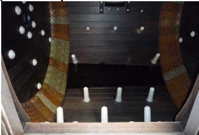
Pegs fitted in a wooden drum. (Drain via perforated side channels)
