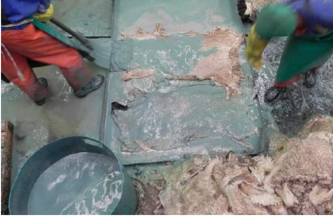
Skins piled to enable “paint” penetration to the hair root.
