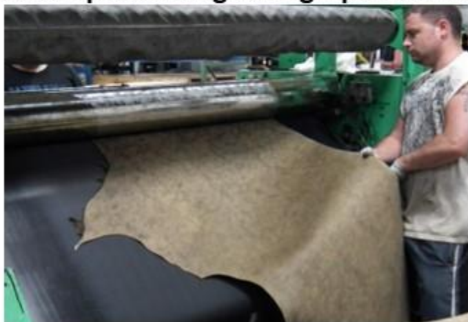
Grain patterning using special rollers.
