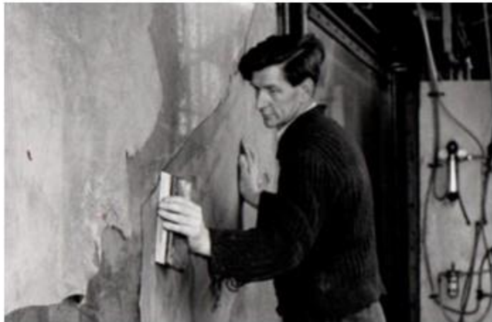
Hand slicking - leather grain to plate.
