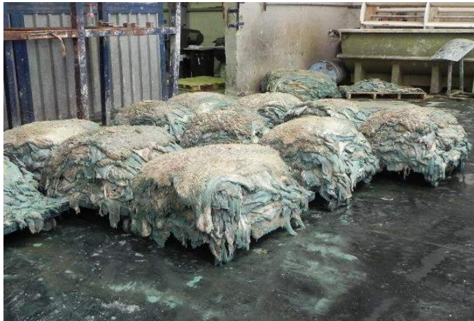
Skins piled to enable “paint” penetration to the hair root.
