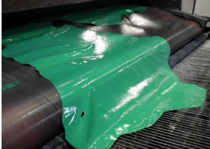
Grain patterning using special rollers.
