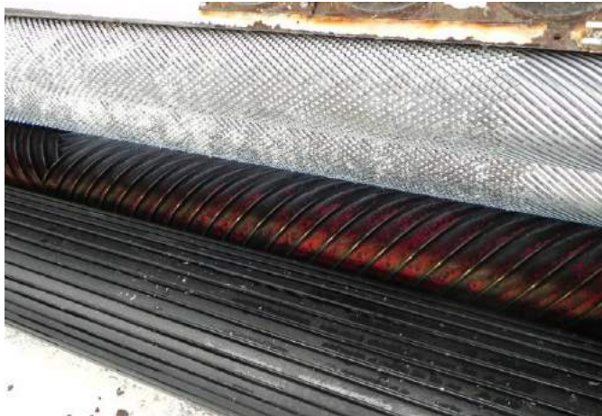
Knife cylinder and transport rollers.
