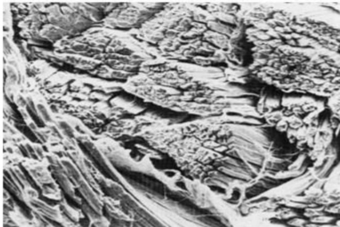
Well separated fibre bundles.
