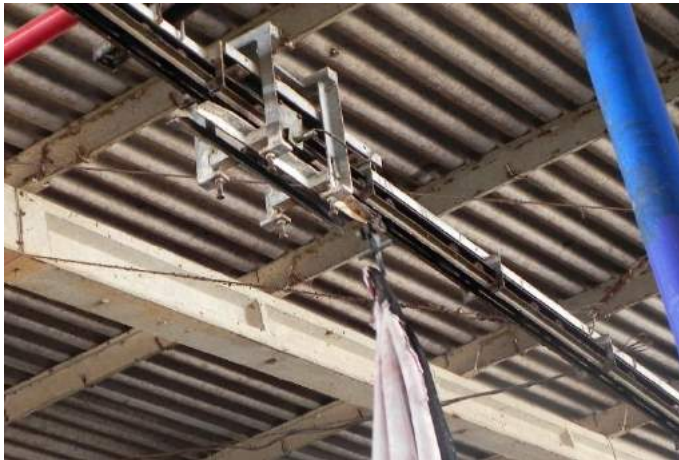
Load cell for weighing each hide.
