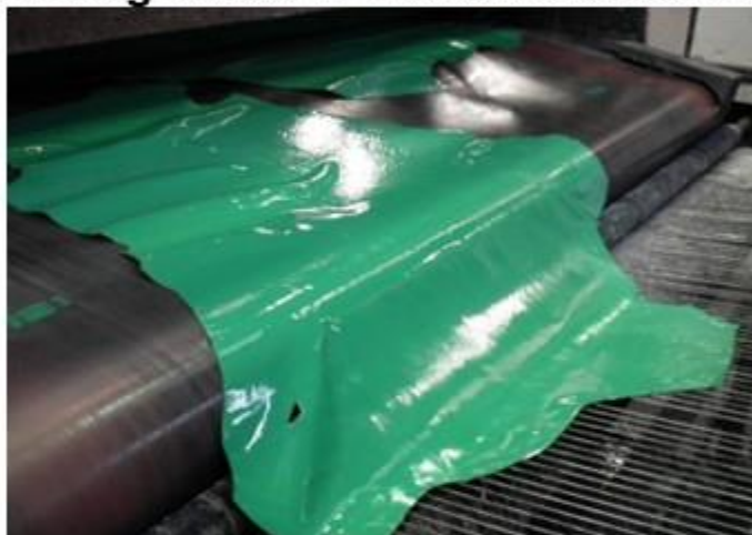
Grain patterning using special rollers.
