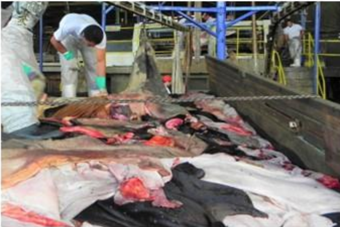
Line-conveyor receipt of fresh hides.
