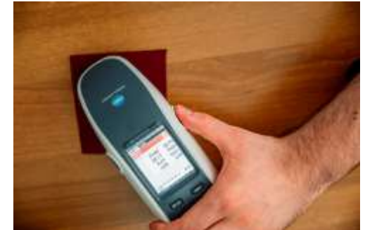
PORTABLE SPECTROPHOTOMETER FOR USE IN THE TANNERY
