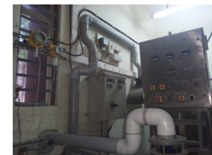
Pictorial view of PLC driven Fabricated dosing system – This figure shows a pictorial skeleton of designed modules of automation at CSIR-CLRI. The unit operations are sequenced and recipe are dosed over time.
