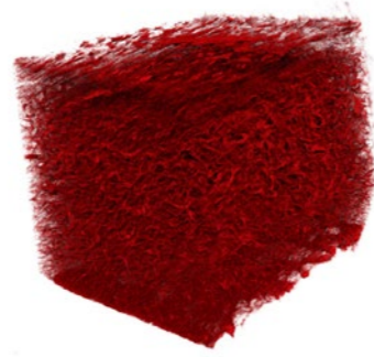
Figure 2 – 3D model of interspace between fiber bundles
