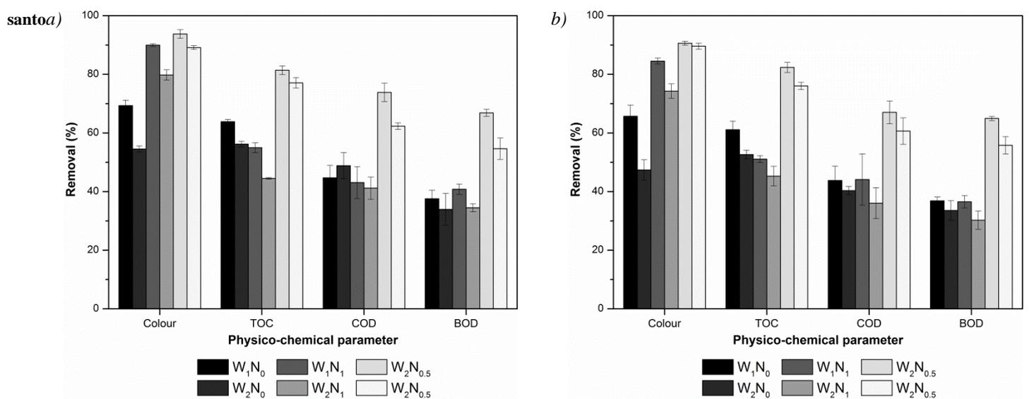
**Figure 3.** Biodecolourization efficiency and mycoremediation after 11 days of treatment with *T. villosa* SCS-10 of wastewaters  $W_1$  and  $W_2$  in the nutrient conditions  $N_1$  and  $N_{0.5}$  for: a) Wastewaters containing Acid Red 357 (W-AR<sub>357</sub>) and b) Wastewaters containing Acid Orange 142 (W-AO<sub>142</sub>).
