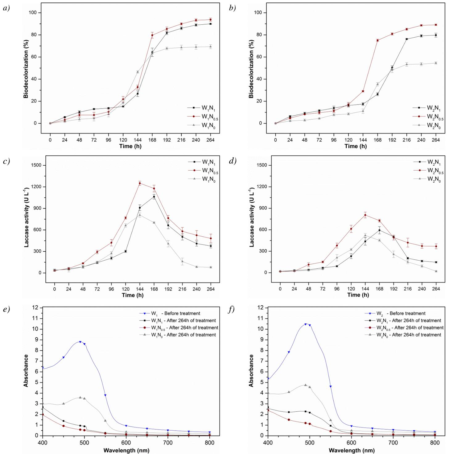
**Figure 1** – Decolourization kinetics of leather dyeing wastewaters containing Acid Red 357 (WS-AR<sub>357</sub>) by a native strain of *Trametes villosa* SCS-10: *a)*  $W_1$  wastewater sample; *b)*  $W_2$  wastewater sample. Laccase activity during the process of decolourization of wastewaters: *c)*  $W_1$ ; *d)*  $W_2$ . UV-Visible spectrum analysis during biodecolourization: *e)*  $W_1$ ; *f)*  $W_2$ . The bars indicate the standard error between three replications.
